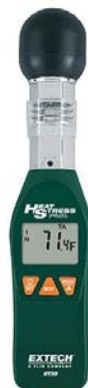
Figure 4. Handheld device with a direct readout of WBGT index (ExTech HT30; http://www.extech.com/display/?id=14523 ).
