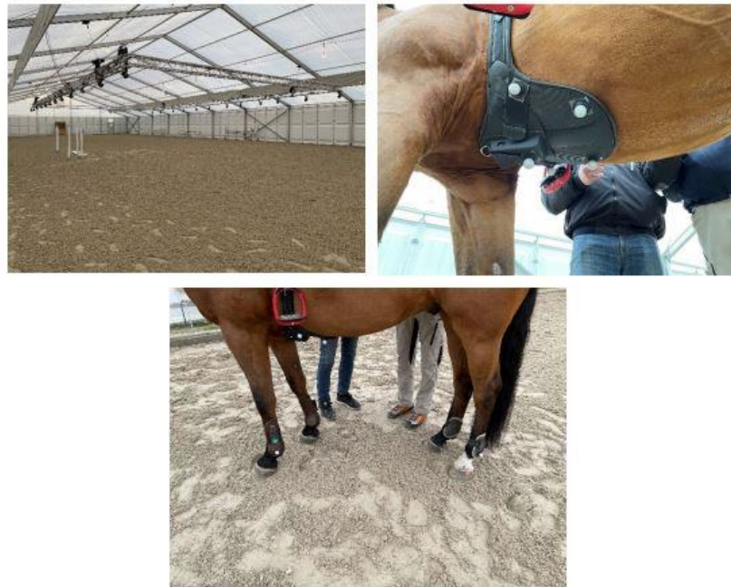
Figure 1. Arena, protective plate with markers, and markers on the brush boots.
